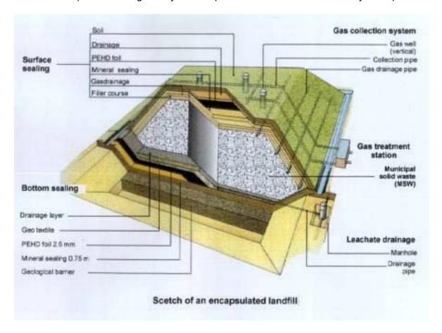
The capsule and the incorporated structures, such as gas and leachate collection systems, manholes, pipes etc., are subjected to stress in view of various influences:
